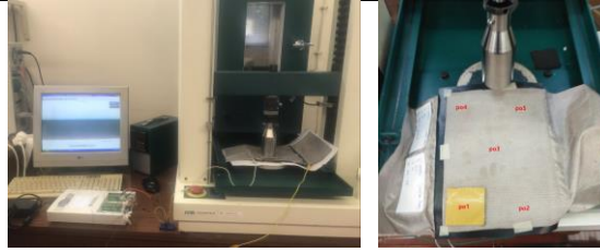
Fig. 5. Setup for compression test (left), testing areas (right)
