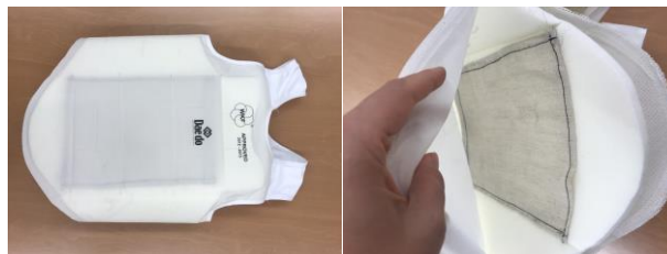
Fig. 2. The unstitched body protector and the pocket sewn inside
