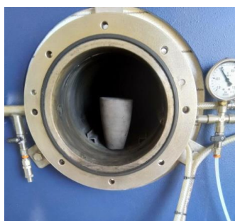
Fig 1. The vacuum furnace used for almost fully reduction of GO.
