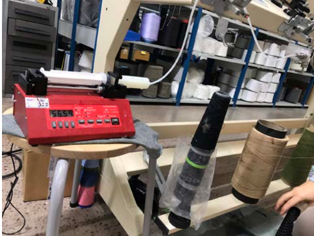
Figure 15: Application of finishing material onto paper yarn
