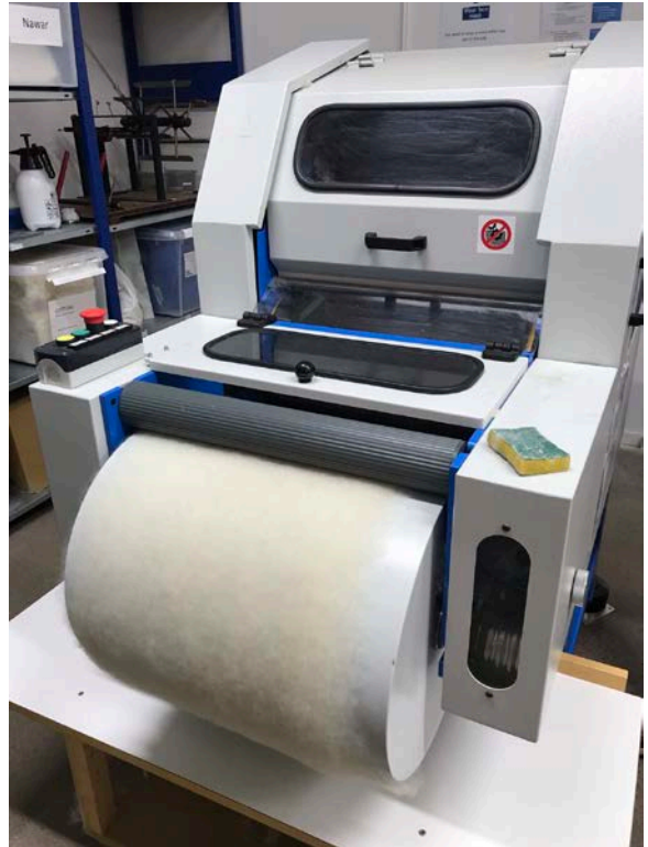
Figure 2: Carding lyocell fibers
