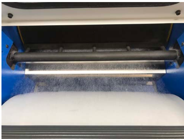
Figure 3: Carding lyocell fibers
